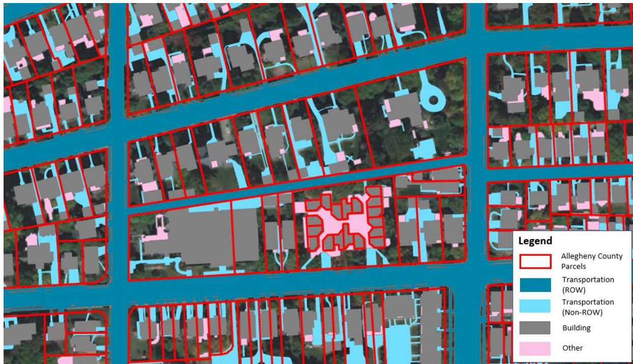
Figure 2. PWSA Transportation, Building, and Other Impervious Data Layers Intersected with Allegheny County Parcel Data to Estimate ROW Impervious
